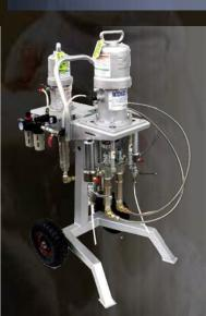
For spraying PU foam application, Paintechnik **SD60-24:1** with mixing ratio 1:1 are designed to overcome the toughest job site environment. Equipped with two positive displacements can provide the most reliable mixing ratio and **COMPACT 6-inch** can always achieve your expectation about fluid atomization.
